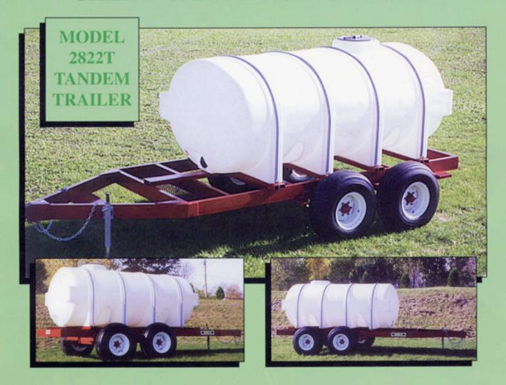
P & H is introducing the latest Model 2822T tandem trailer to add to our line of tandem trailers. The 2822 is built with the same durability & toughness that our other trailers are noted for throughout the industry. It comes with heavy duty leaf springs & equalizer arms which distributes the weight equally over the trailer.
